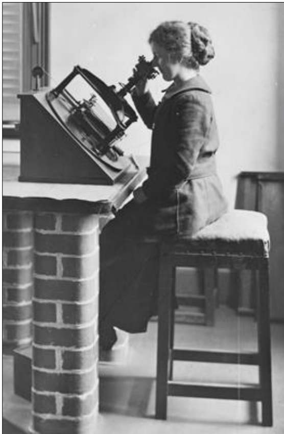
Figure 2: Photograph taken at Melbourne Observatory ca. 1900 showing the Repsold Machine and one of the first women employed as a star measurer and computer (courtesy: Collection Museums Victoria).
