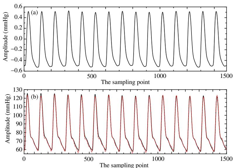
**Figure 10** (Color online) The reconstruction result. (a) Input PPG signals (250 Sample/Second, MIMIC databases 230); (b) the original BP and the reconstruction BP (250 Sample/Second, MIMIC databases 230).
