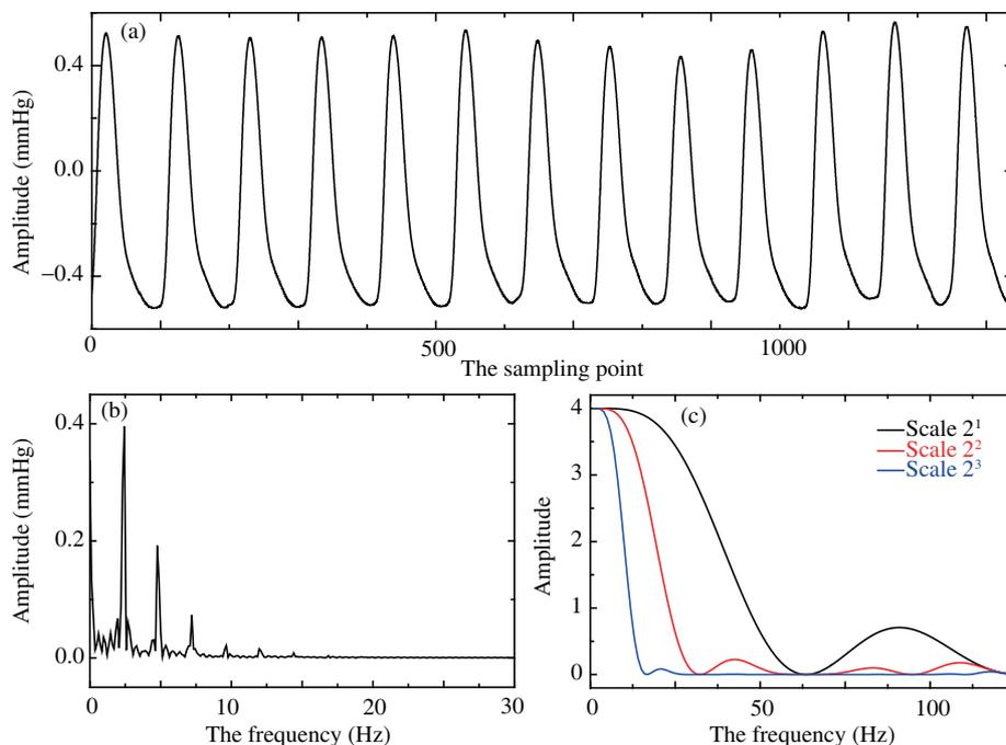
**Figure 4** (Color online) (a) Original PPG signals extracted from MIMIC databases; (b) the FFT spectrum analysis of signals in (a); (c) the frequency response of the Daubechies wavelet at different scales.
