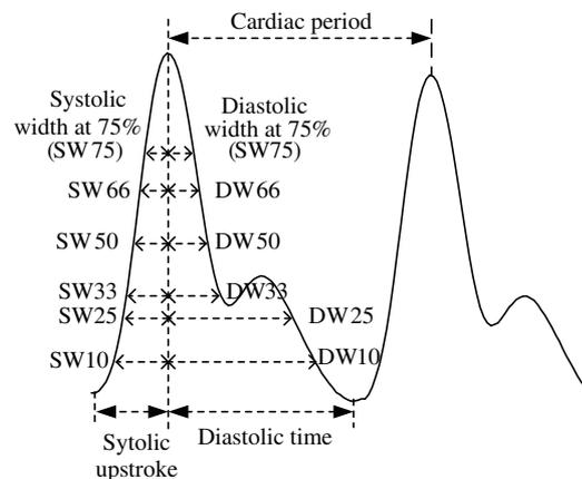
**Figure 2** Multi-feature extraction from a single PPG.
