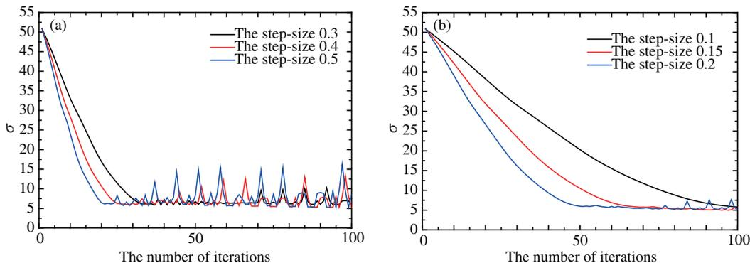
**Figure 7** (Color online) The reconstruction error in different number of iterations. The relationship between the number of iterations and the reconstruction error (Long step-size (a) and Short step-size (b)).
