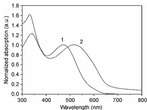
**Figure 2** Absorption spectra of PTh solution in chloroform (curve 1) and PTh film spin-coated (curve 2) from chloroform solution.
