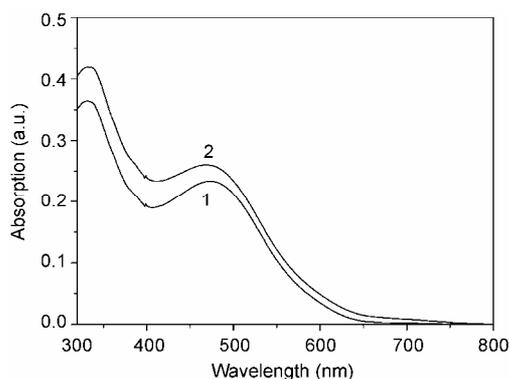
**Figure 3** Absorption spectrum of  $1.0 \times 10^{-5} \text{ g/mL}$  PTh in chloroform (curve 1) in the absence and (curve 2) in presence of  $1.87 \times 10^{-3} \text{ mol/L}$   $\text{TiO}_2$  suspension.
