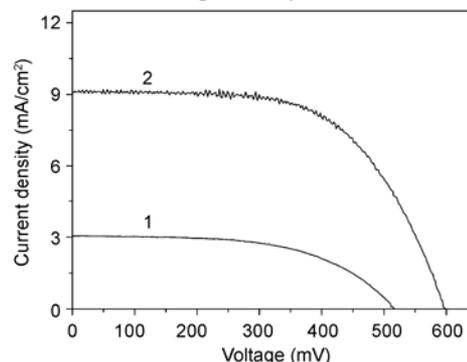
**Figure 7** I-V characteristics of PTh-sensitized solar cell (curve 1) and N3-sensitized solar cell (curve 2). (Electrolyte: tetrabutyl ammonium iodide (TBAI) (0.5 mol/L)/ $I_2$ (0.05 mol/L) in a mixture of PC and EC (1:3, v/v)).
