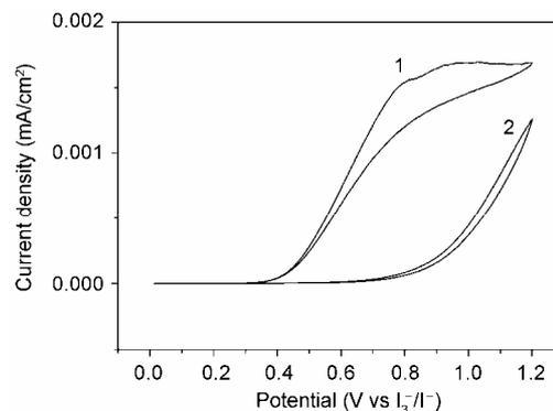
**Figure 8** Cyclic voltammograms of PTh-coated FTO electrode 1 and blank FTO glass 2 measured in the electrolyte containing 0.5 mol/L TBAI, 0.05 mol/L iodine in EC/PC mixed solvent (EC:PC = 3:1, v/v).
