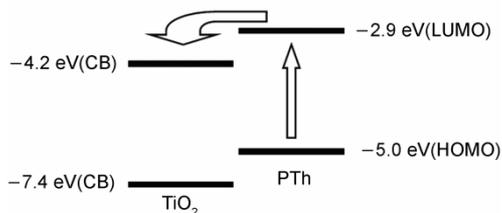
**Figure 5** Schematic energy level of and photoinduced charge transfer at PTh/TiO<sub>2</sub> nanoparticles interface. The vacuum level is defined at 0 eV.
