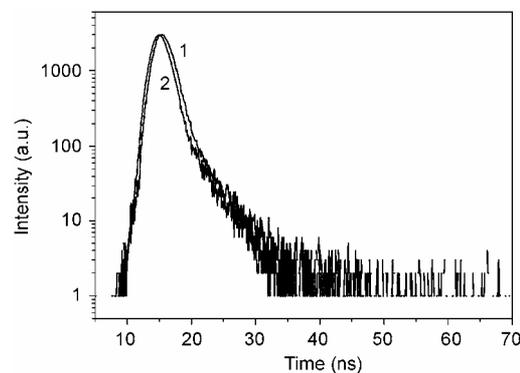
**Figure 6** Fluorescence decay and normalized instrument response curves for  $1.0 \times 10^{-5}$  g/mL in  $1.8 \times 10^{-3}$  mol/L TiO<sub>2</sub>/chloroform suspension. The excitation wavelength was at 471 nm, and the fluorescence emission was recorded at 584 nm. Curve 1 is the fluorescence decay curve fit to a two-exponential decay law and curve 2 is the instrument response.
