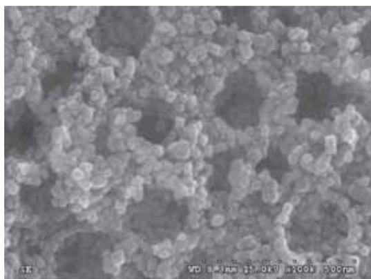
**Figure 1** Surface morphologic image of the nanocrystalline TiO<sub>2</sub> porous film.
